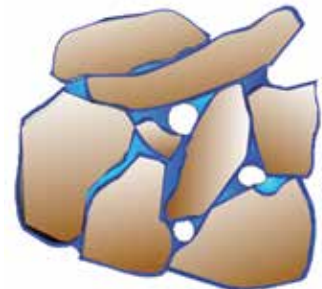
Figure 5.3. A moist sand with pores between grains that contain water and air. The larger pores have partially drained and allowed air entry, while the narrower ones are still filled with water.
