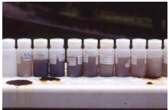
Figure 17.21. Water samples taken from a subsurface drain line when heavy rainfall followed liquid manure application. From left, water samples represent 15-minute sampling intervals from the onset of drain discharge. Photo by Larry Geohring.
