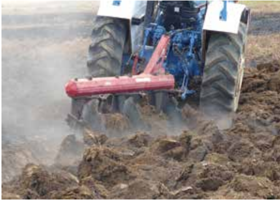
Figure 16.4. Left: A heavy disk (disk plow) can be used for primary and secondary tillage (photo by Mark Brooks). Right: A finishing disk.
