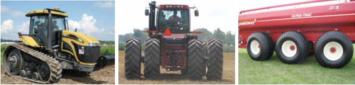
Figure 15.7. Reduction of soil compaction by increased distribution of equipment loads. Left: Tracks on a tractor. Middle: Dual wheels on a tractor that also increase traction. Right: Multiple axles and flotation tires on a liquid manure spreader
