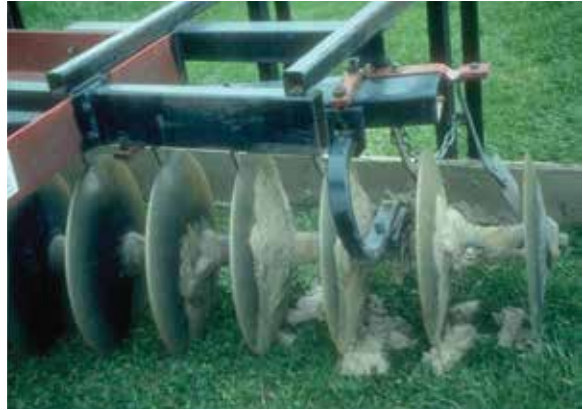
Figure 16.4. Left: A heavy disk (disk plow) can be used for primary and secondary tillage (photo by Mark Brooks). Right: A finishing disk.
